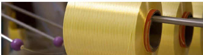
Polyethylene yarn for the production of nonwoven fabrics
