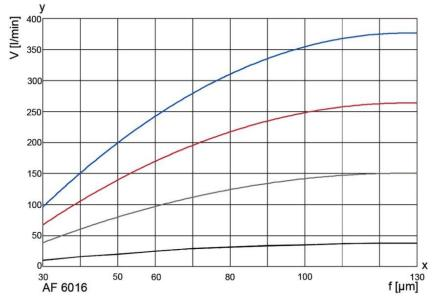
The curves indicate the volume flow through the complete filter system (filter housing including cartridge) and are referred to a differential pressure of 0.3 bar. Specific process information is essential to guarantee reliable operation of an automatic filter.
