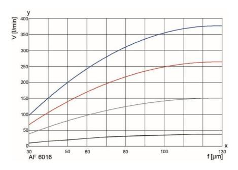
The curves represent the volumetric flow through the entire filter system (filter housing including for example one cartridge) and refer to a differential pressure of 0.3 bar. Specific information about process data is essential for reliable operation of an automatic filter.
