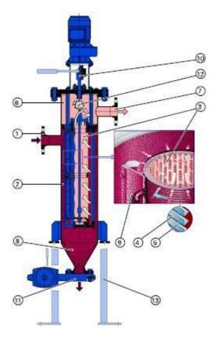
The filtered fluid exits the filter housing at the top opposite the inlet connection. In the AF 94 S version, the integrated preseparator relieves the filter cartridge of coarse and heavy particles by means of a tangential flow around the tube.
