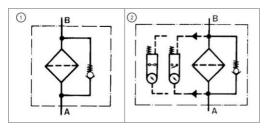
Bypass valve is integrated into the filter element.
